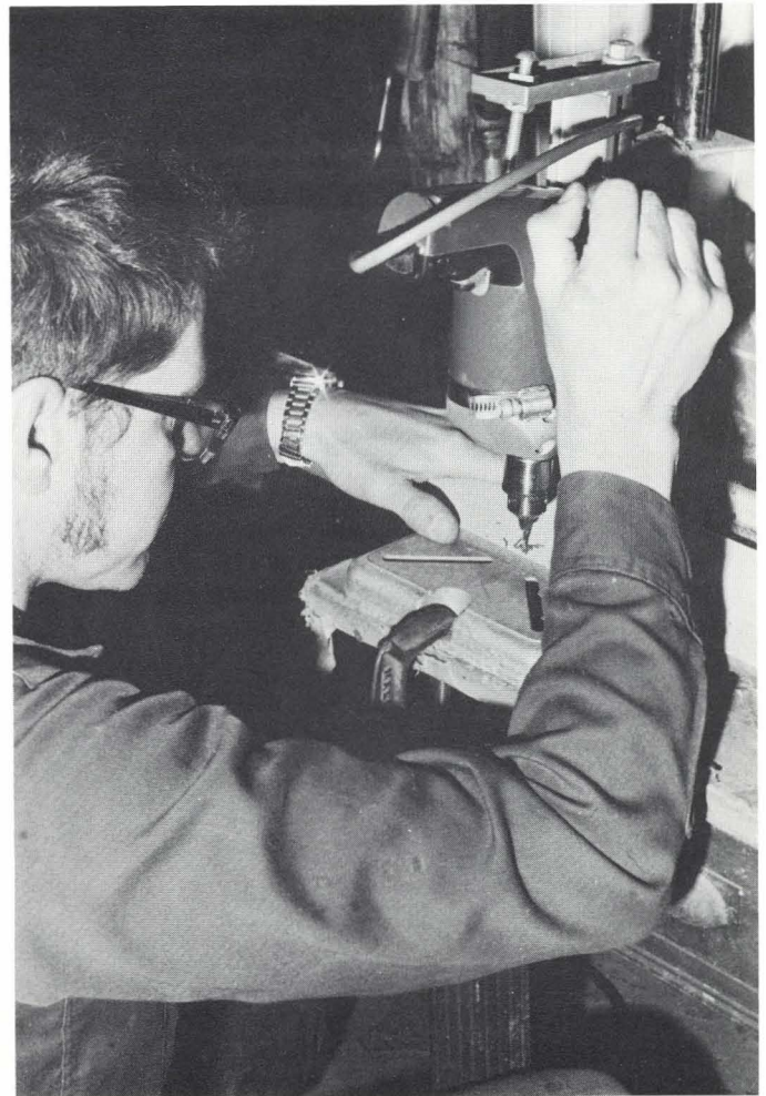
It is necessary to predrill nail holes in the hardboard for assembly.
